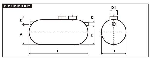
All dimensions are in millimetres. Units.>NS 20 have multiple necks fitted. Units >NS 80 have multiple coalescers
